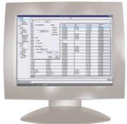
Capacity planning reports project historical traffic trends to user-specified thresholds, or to a future date. Engineers can easily identify which links need to be upgraded, and when, as well as examine projected link traffic by CoS, customer or ingress/egress PE router.
