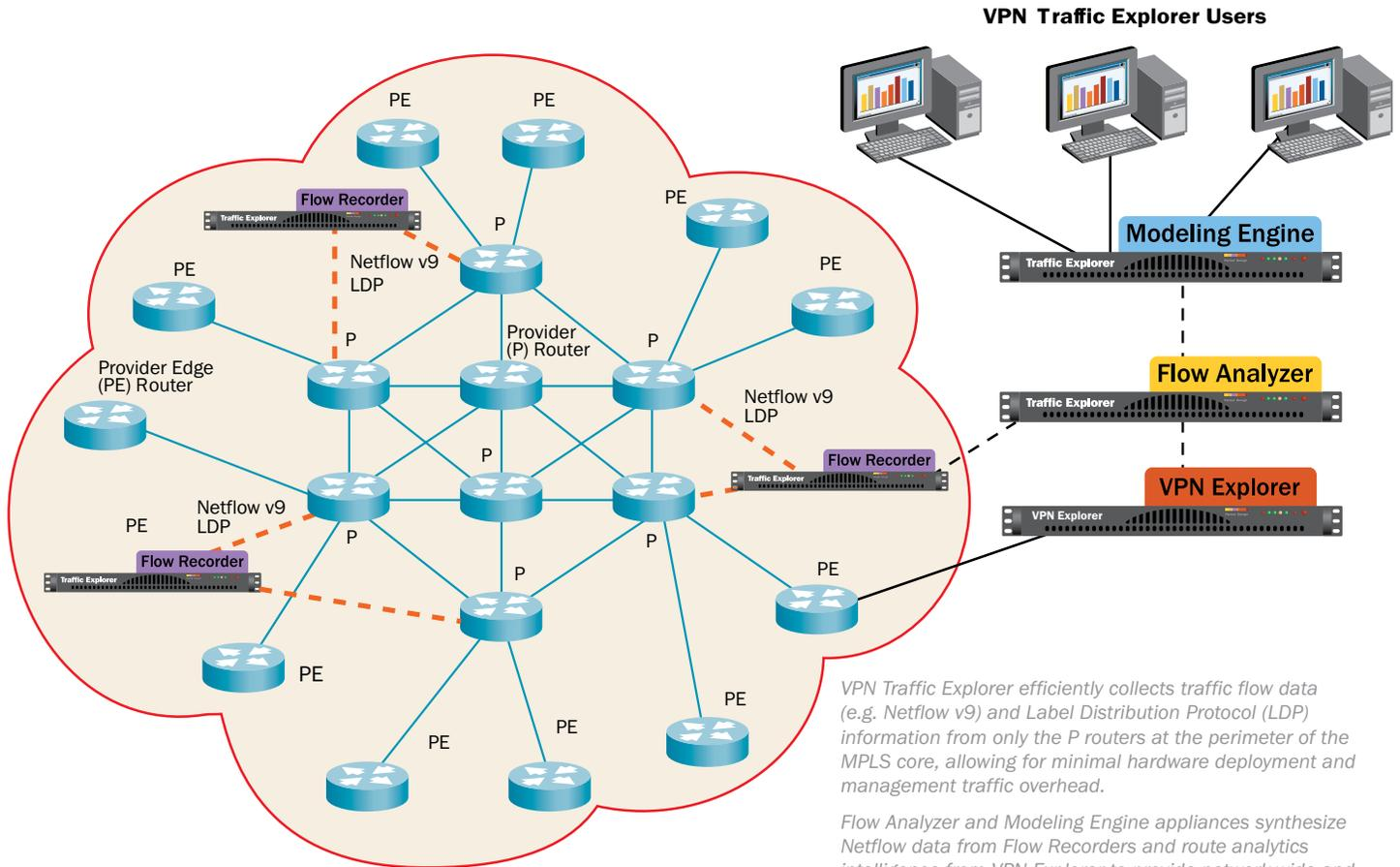
VPN Traffic Explorer efficiently collects traffic flow data (e.g. Netflow v9) and Label Distribution Protocol (LDP) information from only the P routers at the perimeter of the MPLS core, allowing for minimal hardware deployment and management traffic overhead.
