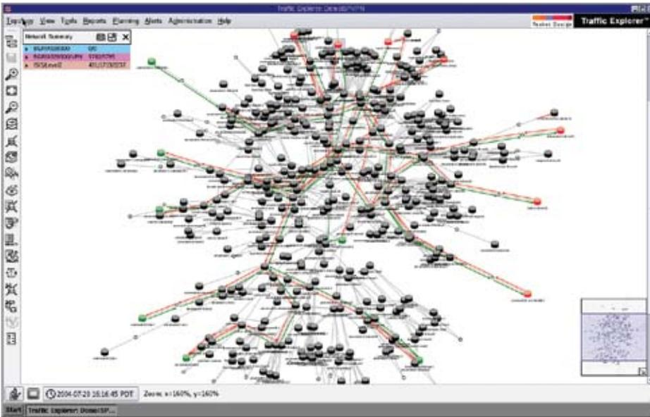
VPN Traffic Explorer provides a view of the service provider's entire network topology. Operators can monitor and analyze aggregate, per-CoS and per-customer traffic on all links in the network. Engineers can view complete, end-to-end paths connecting customer sites, and drill down to routing and traffic details on any link or node.
